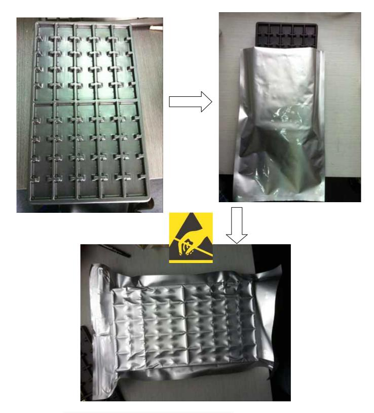
Pumping air into vacuum state, anti-static packaging
