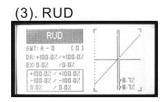
Dual rate is to adjust aileron, elevator and rudder travel range. The range is between 0%-120%.
