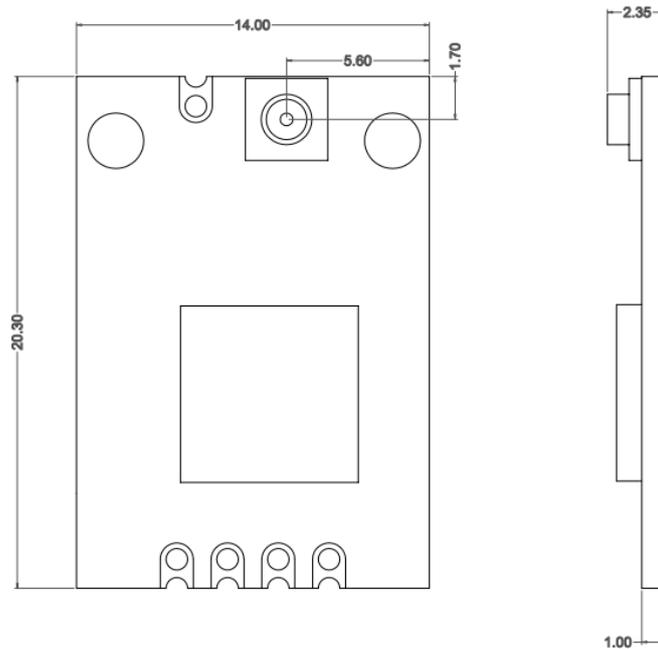
Module dimension: 20.3\*14.0\*2.35mm(L\*W\*H; Tolerance: ±0.15mm)
