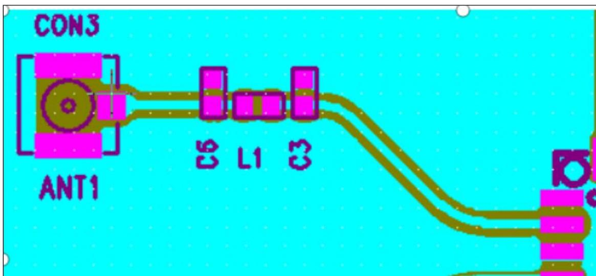
The module needs to be attached to the PCB board and connected to the external antenna through the solder joint of the circuit on the PCB. The gain of the external antenna is 2dBi (Max.)
