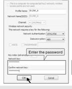
Note: The password should be the same as which set on the router or AP
