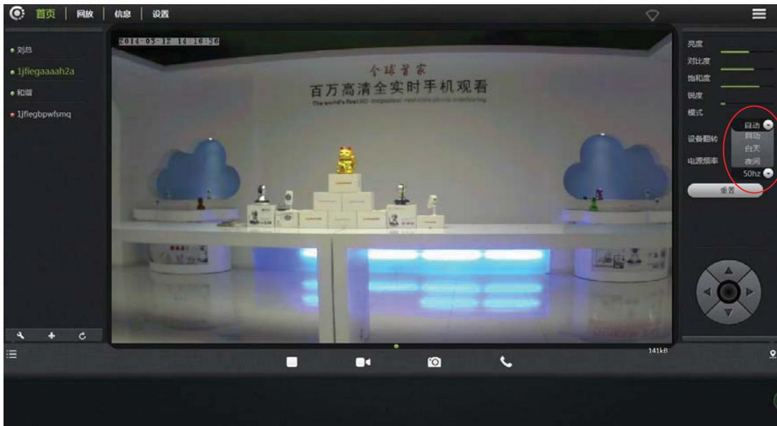
1. Automatically: Infrared lamp's on and off is based on the environment around the photosensitive sensor.
