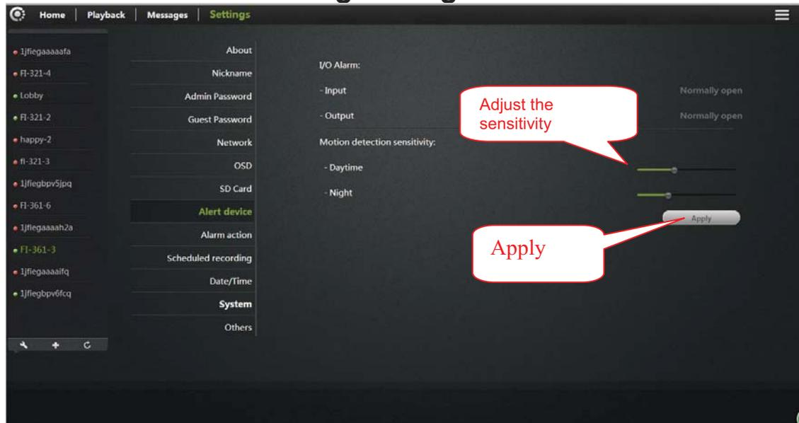
**I / O Alarm input:** When normally open, alarm input port connect with an external alarm sensor (such as door sensor, infrared, smoke alarm detector, etc.) must be a normally open alarm probes. When alarm occurs, the probe switch is closed; network cameras generate alarm triggers, alarm calls according to user settings.
