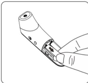
2. Take the probe cover off from the thermometer before measuring the ear temperature.
