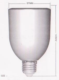
Power: Speaker 10 W, LED 5W (600-800LM) Speaker :  $8\Omega$  10W Interface : E27 Amplifier : Class D Signal input: Bluetooth. 2.4G Bluetooth transmission Bluetooth transmit distance : 10 meters Bluetooth connection password : 0000 Signal output : 300-15K audio signal Working temperature : -40°C~80°C Working voltage : AC100-240V Life : >40000 hours
