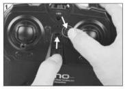
按下升降微调向上键不放的同时打 开电源开关,待提示音结束后松开, LED灯亮起,中立点复位; Press and hold the button CH2 UP, turn on the transmitter, then the LED light will be on. The neutral position of the control stick resets.
