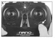
快速按下并松开副翼微调向右键按钮, LED指示灯亮起,中立点复位; Press the button CH1 DOWN, then the LED light will be off.
