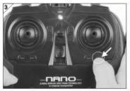
快速按下并松开副翼微调向右键按 钮,LED指示灯熄灭,中立点复位; Press the button CH1 DOWN quickly, and then the LED light will be off. The neutral position of the control stick resets.
