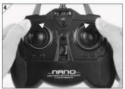
轻摇发射机摇杆后,再将摇杆置中; Lightly push the throttle stick, and then center it.
