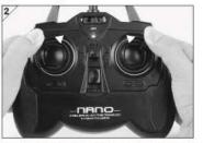
最大范围地摇动发射机摇杆两到三次, 再将摇杆置中; Roll the throttle stick to the maximum
