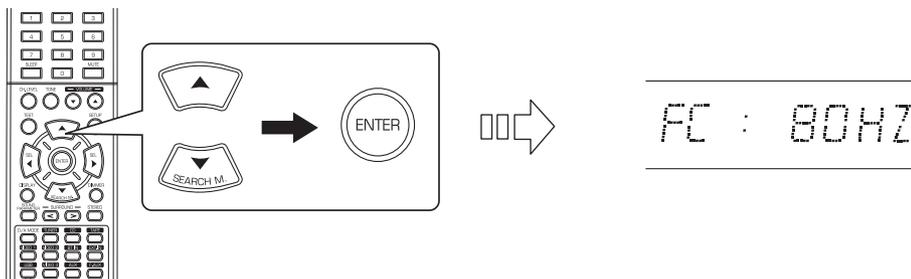
2. Press the CURSOR LEFT(◀)/RIGHT(▶) buttons to set the crossover frequency as desired.
