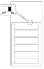
Activate the "False Alarm/Initial Warning" mode by opening the battery door and removing the batteries on the Siren Main Unit. Flip the "Delay" switch into the ON position and replace the batteries and the door. Press the OFF button of the Key Chain Remote. The Siren Base Unit should beep once, showing it is set up and ready to use.
