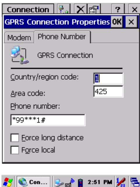
Figure A-21 Set GPRS Connection-Phone Number
