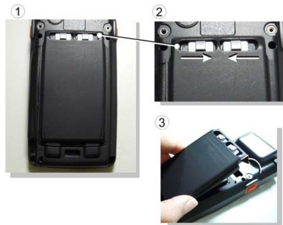
Figure 2-4 Detach the battery cover from Device
