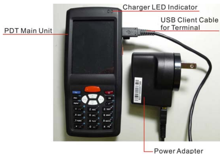
Figure 2-7 Charging with power adapter
