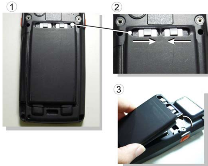
Figure 2-18 Detach the battery cover from Device
