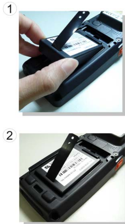
Figure 2-5 Insert the battery pack
