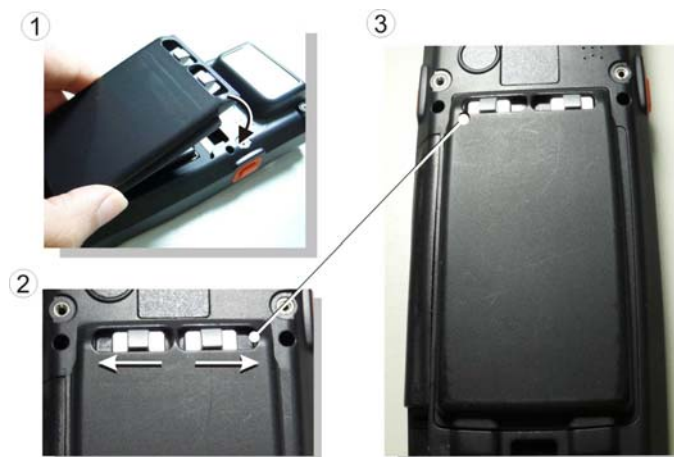
Figure 2-6 Replace the battery cover
