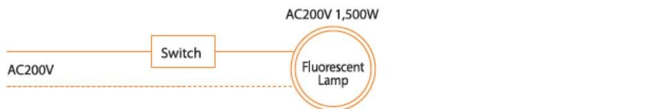
[ General Wiring of Fluorescent Lamp ]
