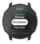
To shutdown your G5, unlock the watch and navigate to the main menu from the clockface screen.
