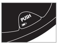
Low Power Indicator Steady Red: Power low. Replace batteries immediately
