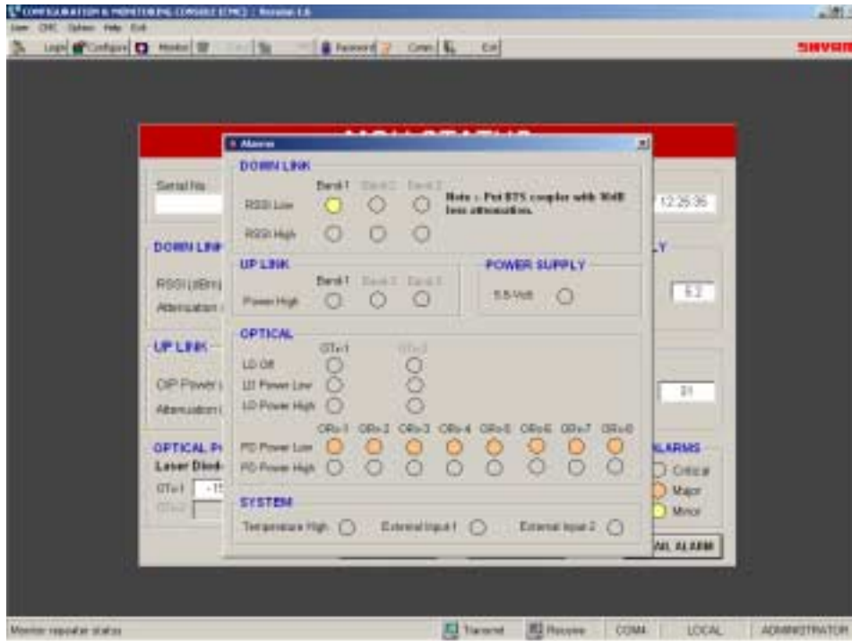
Figure 6: MOU Alarm Monitoring
