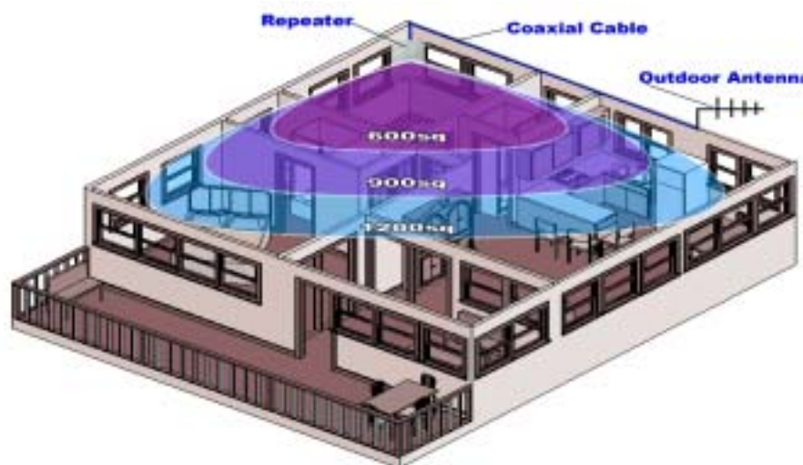
Figure 1: Typical Repeater/Coverage Configuration
