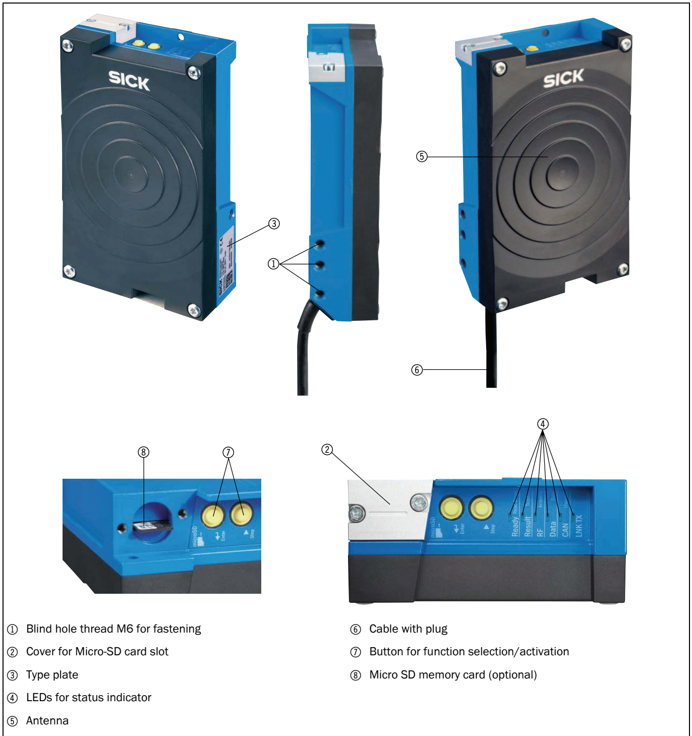
Fig. 4-1: Device view of the interrogator RFH620 (standard version)
