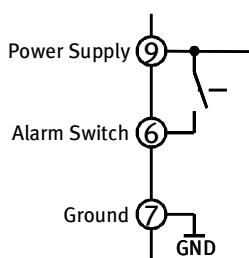
Output Voltage: 0 (disabled) or Power Input Voltage (enabled)
