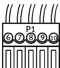
5-pole connector with clamping screw
