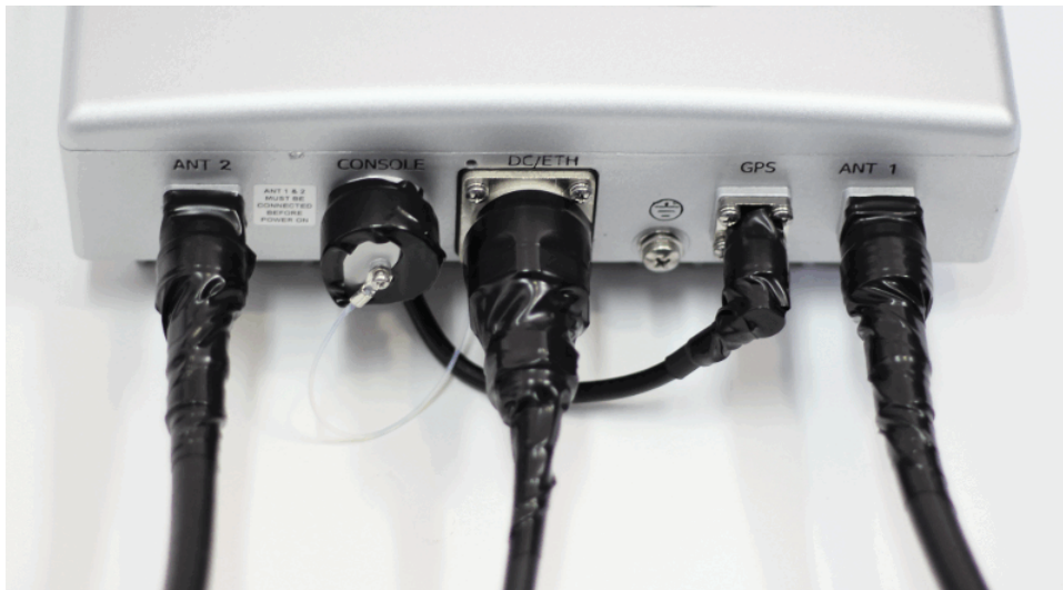
Figure 23: Base Station Connectors wrapped with Splicing and Electrical Tape
