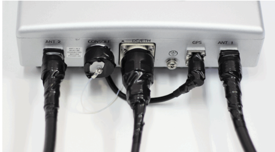
Figure 4.14. Base Station Connectors wrapped with Splicing and Electrical Tape
