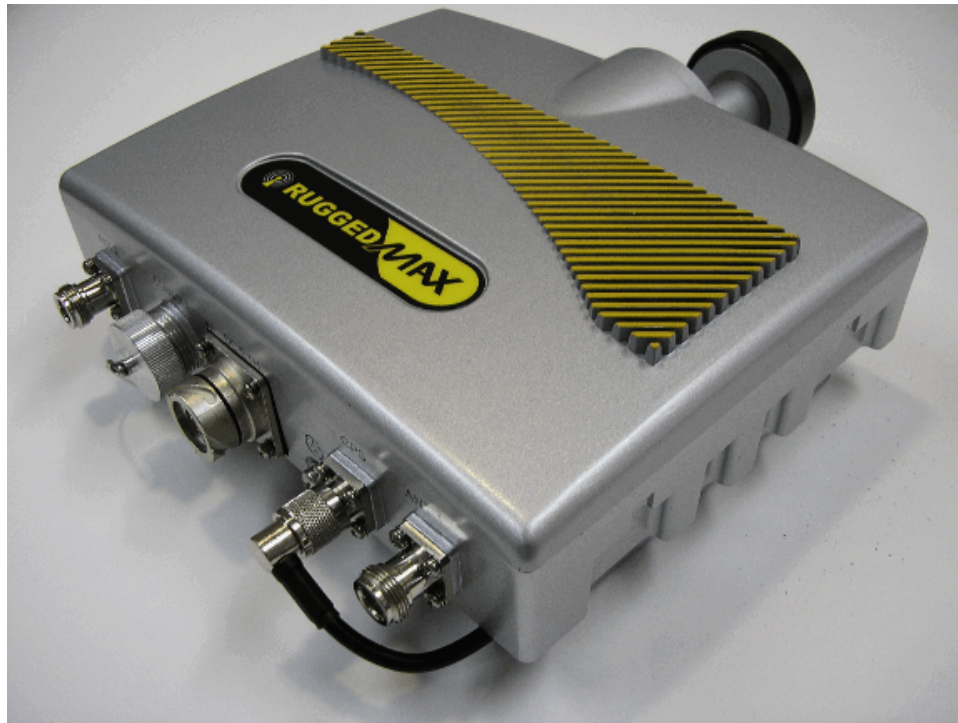
Figure 2.1. WiN7200 Small Form Factor Base Station
