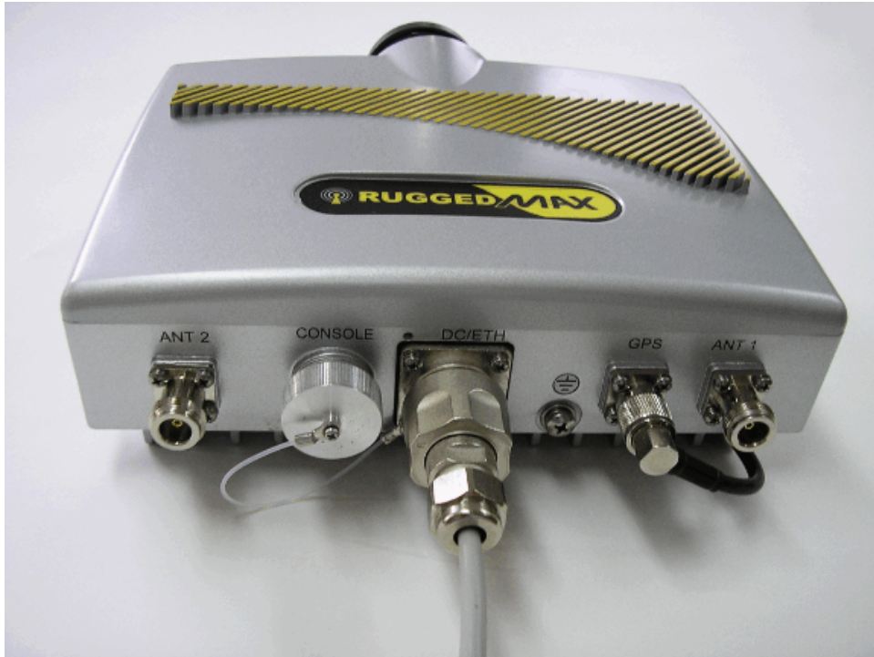
Figure 4.8. PoE connector secured to base station
