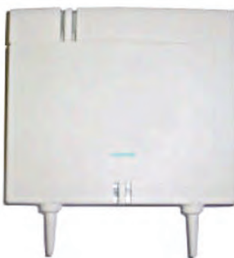
Figure 6 DECT IP base station BSIP1 (Item number: U30807-S5494-X)
