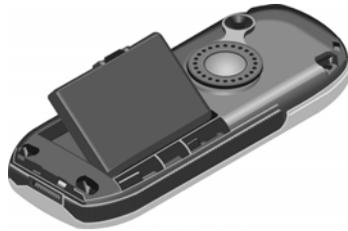
5. Hold the battery cover at a slight angle and insert the two projections provided on the lower side into the battery compartment. Then close the cover until it snaps shut.
