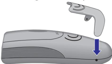
Push the belt clip onto the back of the handset until the lugs at the side click into place.
