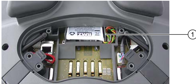
① Cable routing
