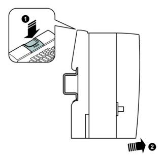
Follow the steps below to remove the SCALANCE W760/W720 from a DIN rail:
