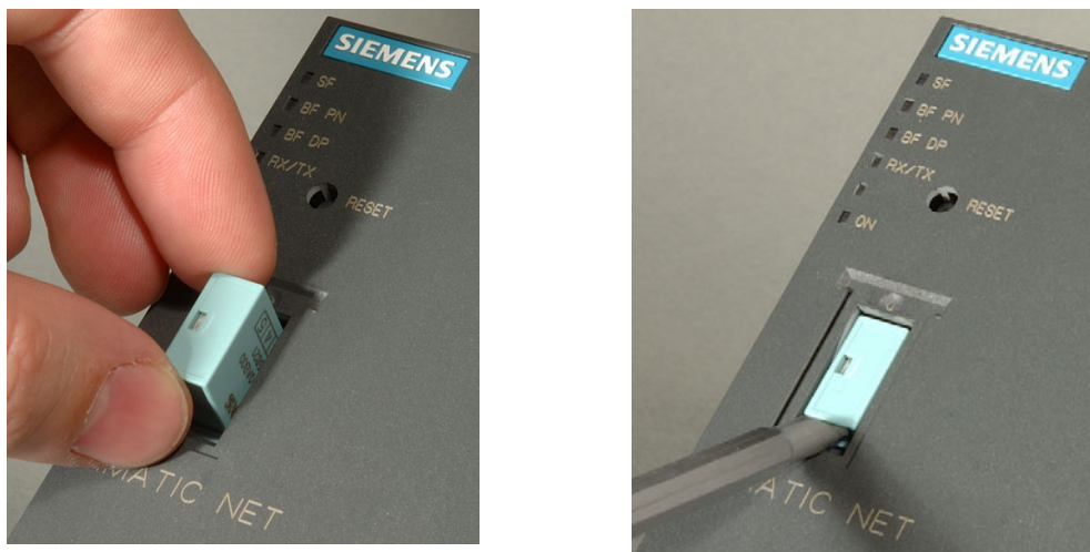
Figure 2-3 Fitting a C-PLUG in the IWLAN/PB Link PN IO and Removing a C-PLUG from the IE/PB Link PN IO using a Screwdriver
