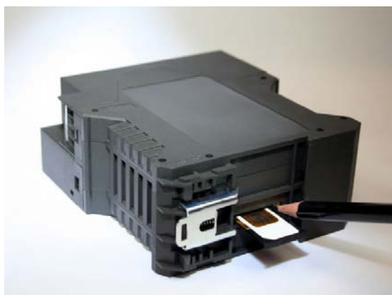
Figure 2-3 Inserting the SIM card
