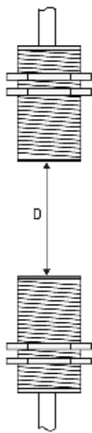
Figure 6-33 Face-to-face distance between two ANT 18s
