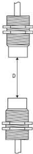
Figure 6-38 Face-to-face minimum distance between two ANT 18 (stainless steel variant)
