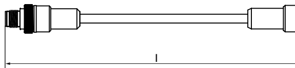
Figure 7-54 Connecting cable/extension cable M12 ↔ M12; l = 2 m, 5 m, 10 m, 20 m, 50 m
