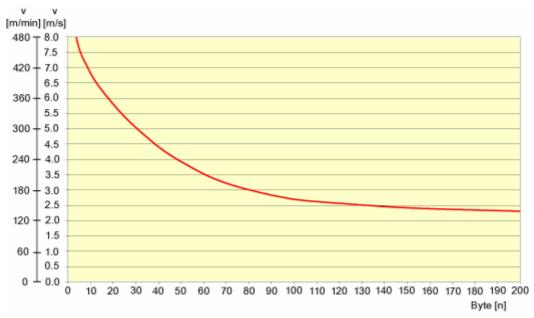
Figure 4-17 Relationship between speed and volume of data (reading/writing from FRAM) in dynamic operation when using the RF350R with ANT1 and RF320T
