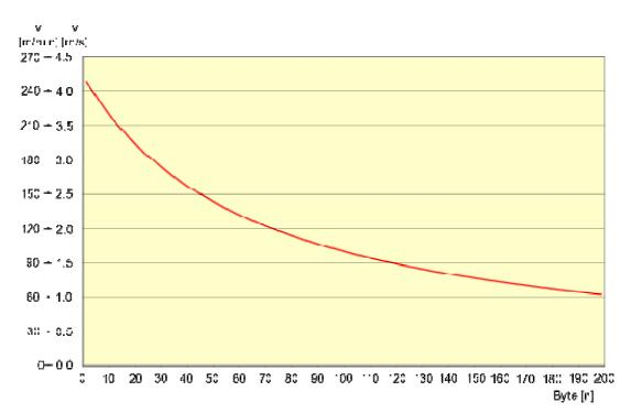
Figure 4-12 Relationship between speed and volume of data (reading/writing) when using the RF310R (RS 422) and RF350T/RF360T
