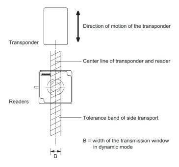
Figure 4-7 Tolerance of pallet side transport
