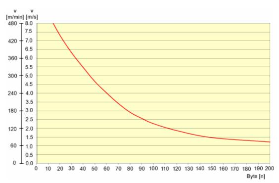
Figure 4-18 Relationship between speed and volume of data (reading/writing from FRAM) in dynamic operation when using the RF350R with ANT1 and RF340T
