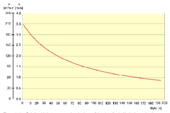
Figure 4-11 Relationship between speed and volume of data (reading/writing) when using the RF310R (RS 422) and RF340T
