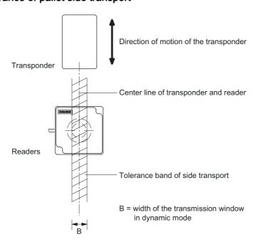
Figure 4-5 Tolerance of pallet side transport
