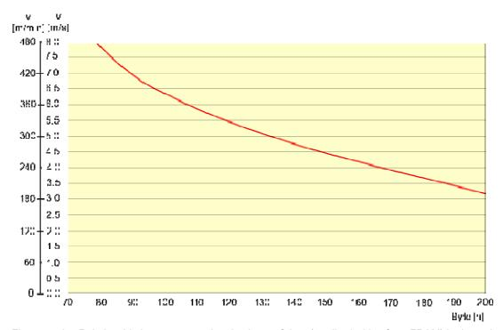
Figure 4-16 Relationship between speed and volume of data (reading/writing from FRAM) in dynamic operation when using the RF340R and RF360T
