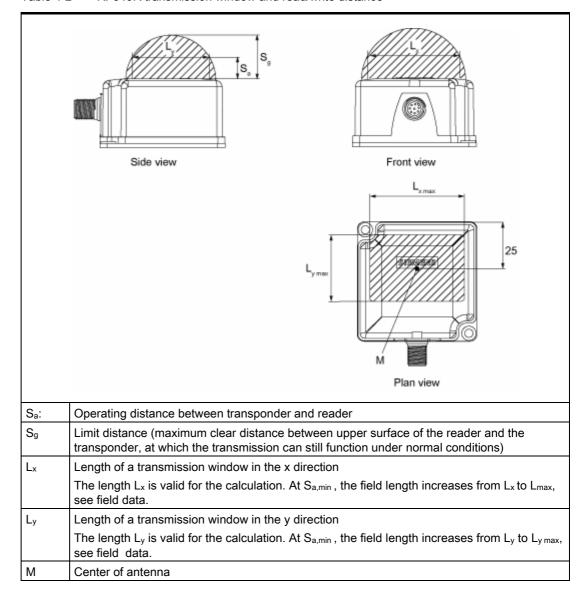
Table 4-2 RF340R transmission window and read/write distance
