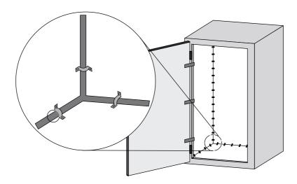
Figure 4-23 Shielding by enclosure
