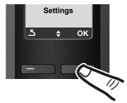
▶ Press the bottom of the control key ↓ until the Settings menu item appears on the display.
