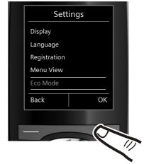
▶ Press down on the control key with until the Eco Mode menu appears on the display.
