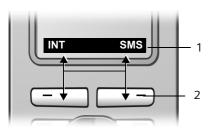
The display keys' current functions are shown in the bottom display line.
