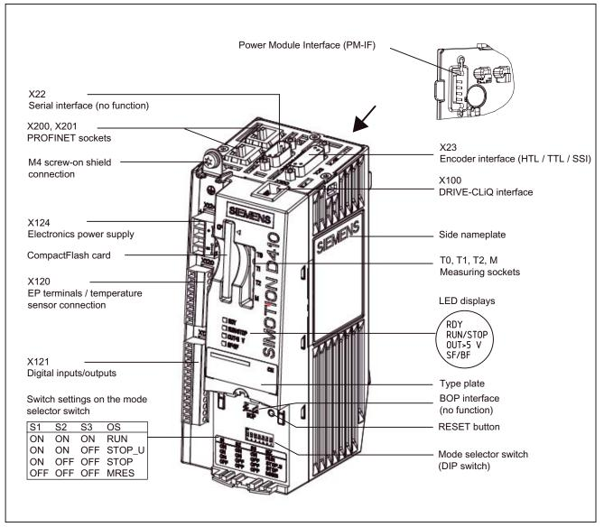
Figure 1-5 Location of interfaces and front elements in SIMOTION D410 PN
