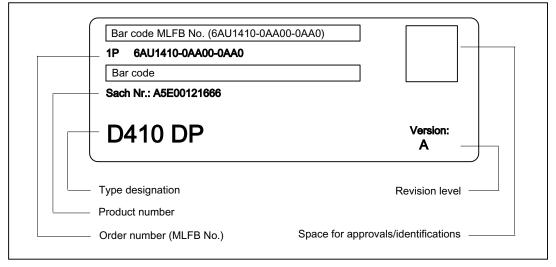
The following nameplate includes the SIMOTION D410 DP barcode numbers and is located on the front side of the module.
