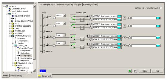
Figure 4-21 Configuring DI/DOs as input or output
