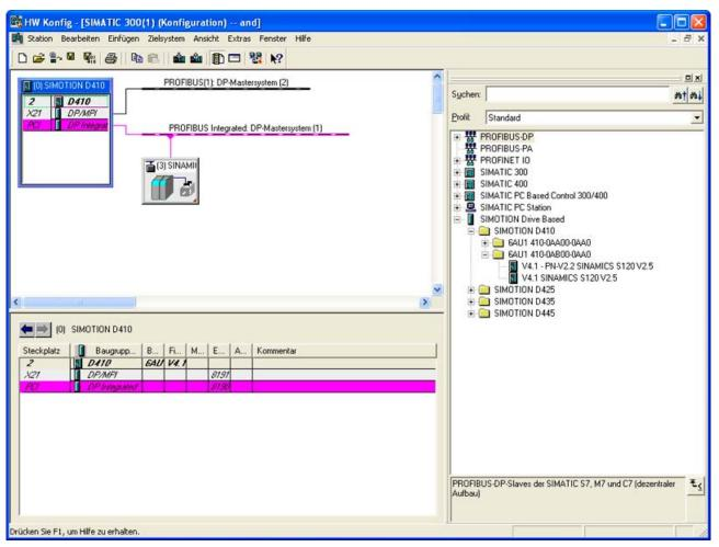
Figure 5-1 HW Config module replacement
