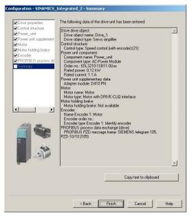
Figure 4-9 Finishing the drive
