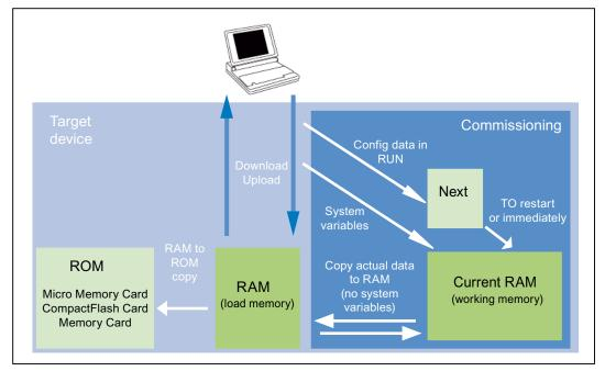
Figure 2-3 Configuration data and system variables on volatile memory
