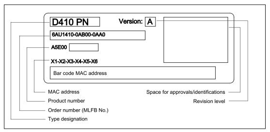
Figure 1-7 SIMOTION PN nameplate (example)
