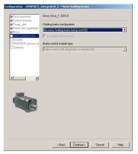
Figure 4-6 Selecting a motor holding brake
