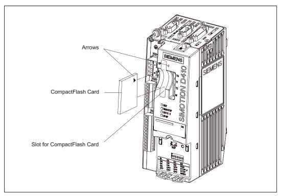
Figure 2-1 Inserting the CompactFlash Card
