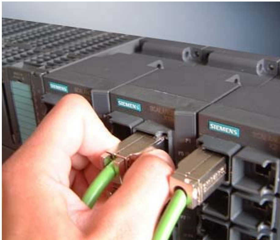
Figure 5-6 Releasing the RJ-45 Plug
