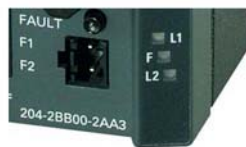
Figure 4-15 SCALANCE X204-2 Signaling Contact
