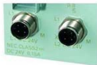
Figure 4-8 SCALANCE X208PRO Power Supply
