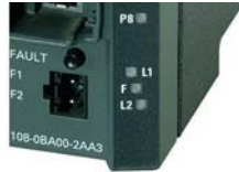
Figure 4-3 Signaling Contact SCALANCE X108
