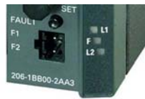
Figure 4-12 SCALANCE X206-1 Signaling Contact
