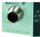
Figure 4-9 SCALANCE X208PRO Signaling Contact
