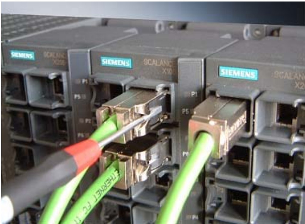
Figure 5-7 Releasing the RJ-45 Plug with a Screwdriver
