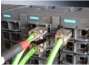
Figure 5-5 Releasing the RJ-45 Plug with a screwdriver
