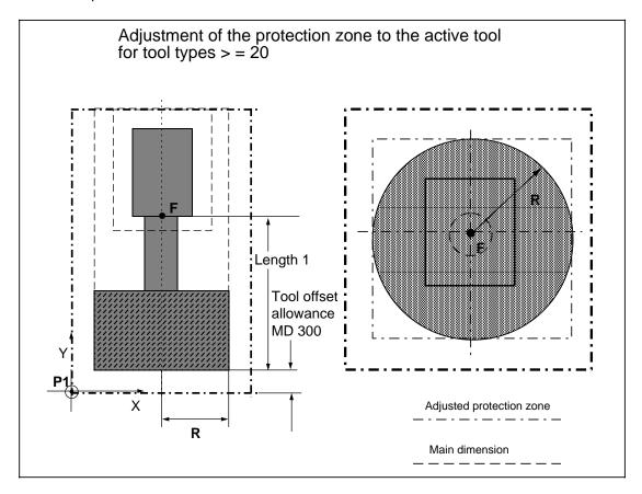
The "protection zone adjustment active" signal is set in the PLC interface DB 48, DW 75 and DW 77 when the protection zone dimensions are set larger than those specified in the machine data. Protection zone adjustment may have been implemented via automatic protection zone adjustment to the active tool (G181 and D number) and/or via the protection zone specific setting data for the additive protection zone adjustment. Differentiation is not possible at the PLC interface.
