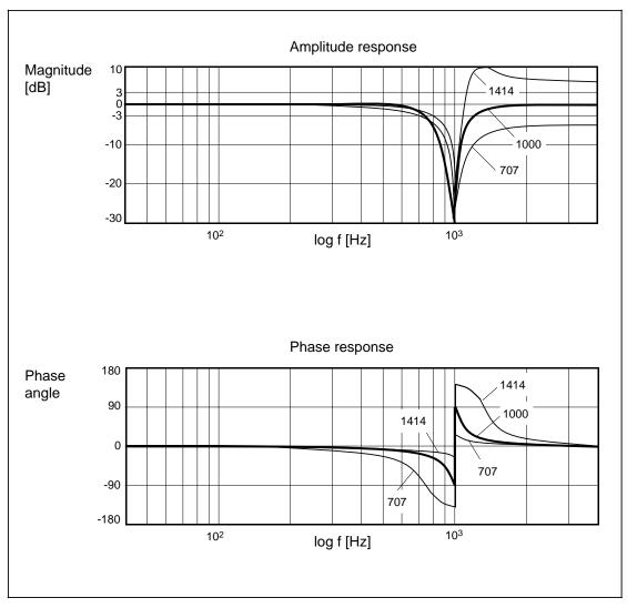
Fig. 12-9 Frequency response of general bandstop with blocking frequency  $f_z = 1000$  Hz, bandwidth  $f_{Bn} = 500$  Hz, counter bandwidth  $f_{Bz} = 0$  Hz and variation in natural frequency  $f_n = 707$ , 1000 and 1414 Hz.
