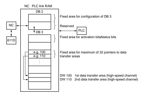
Functional structure of high-speed data channels
