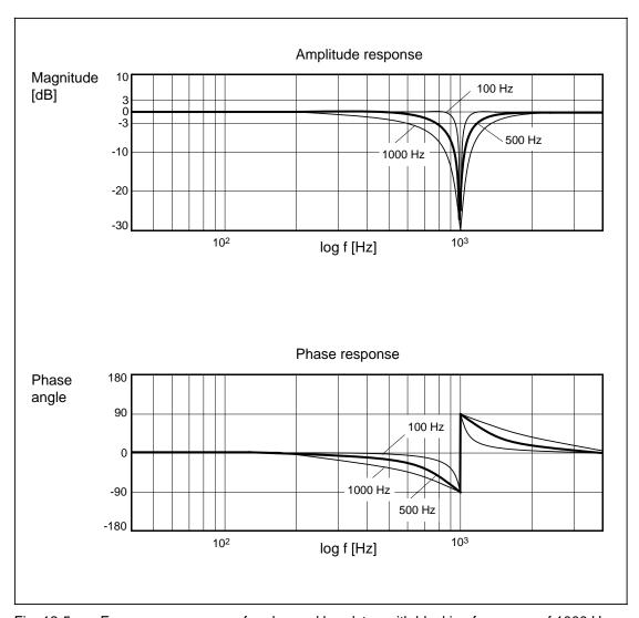
Fig. 12-5 Frequency response of undamped bandstop with blocking frequency of 1000 Hz and bandwidth variations of 100 Hz, 500 Hz and 1000 Hz.
