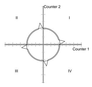
Figure 3 Radius deviations at the quadrant crossover points with insufficient compensation
