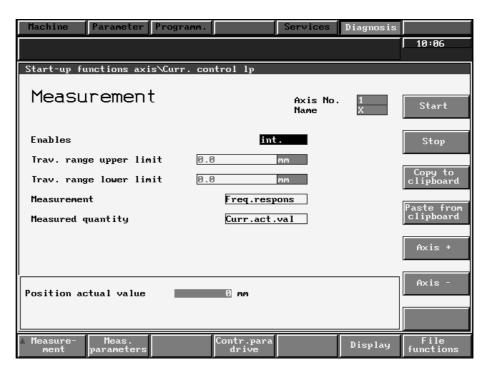
Fig. 9.2 Measuring in a current control loop for axes
