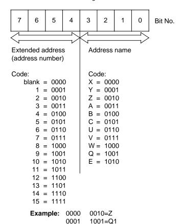
The names in MD 5000, MD 5001 and 568\* must not overlap. Identical address names with different address extensions are not regarded as overlaps.
