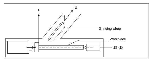
Plain grinding machine with inclined U axis
