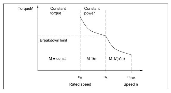
Fig. 1 Torque characteristic of induction motor
