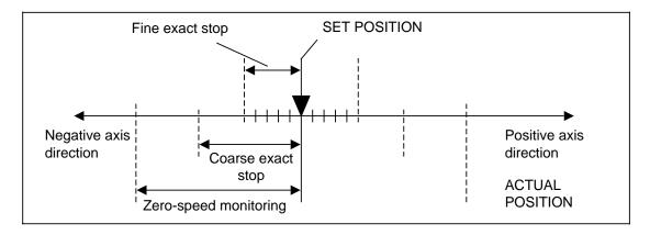
The NC monitors the position at zero speed (holding of position). If the zero-speed monitor is timed out after the waiting time for the position monitor (NC MD 156/NC MD 372\*) has elapsed, alarm 112\* is issued.
