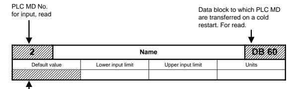
Value initialized when PLC MD are loaded in "Overall Reset" mode
