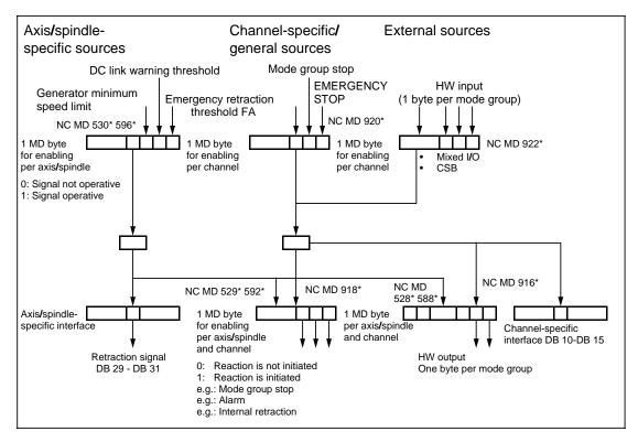
Programmable retraction as open-loop control function
