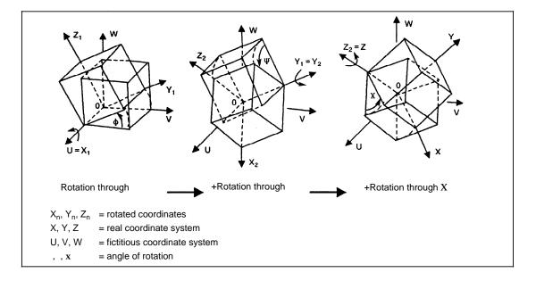
The angle or real machine axis through which the associated axis rotates, is always assigned to the 1st real axis (MD 5065).
