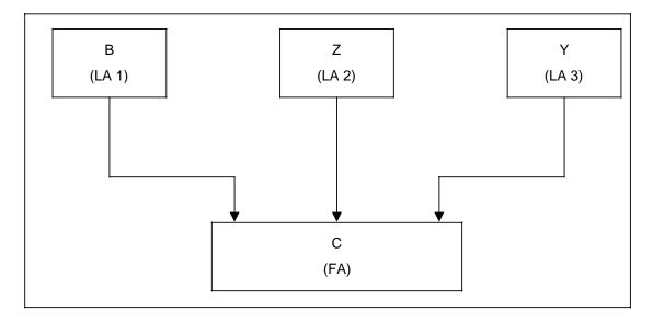
The workpiece table axis (C) is the following axis; in this example, it is influenced by three leading drives.
