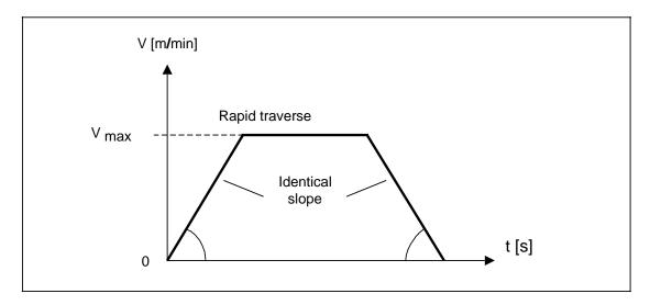
The acceleration values for the axes need not be identical. The control assumes the lowest acceleration value of the interpolating axes involved. These values also apply for deceleration (braking).
