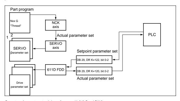
Gear stages/parameter set switchover for axes with 840 C and SW 3
