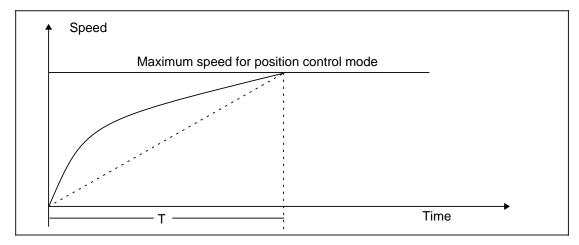
Development of spindle speed in controlled mode at the acceleration limit (M3/M4)
