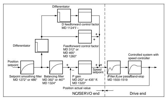
Fig. Position controller structure with filters
