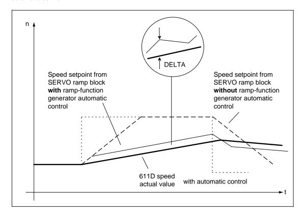
When DELTA is calculated, it must be taken into account that the torque setpoint limitation  $m_{\text{set,limit}}$  may change in cyclic operation. This limitation acts on the maximum speed difference  $n_{\text{max}}$ .
