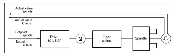
Configuration with two encoders or one double-track encoder
