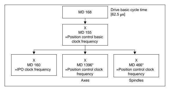
Determination of sampling interval and interpolation time
