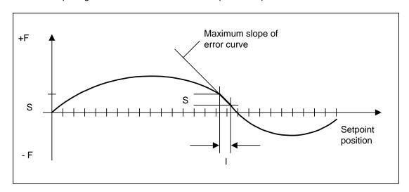
The point with the greatest pitch error is determined and the travel ( I) in which the specified amount ( S) is passed through is established.
