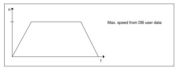
Speed characteristic for incremental positioning
