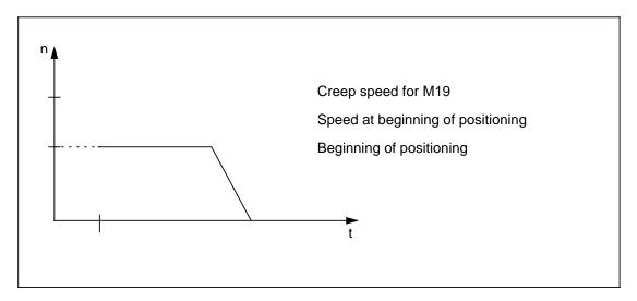
Speed characteristic for case 1b (actual speed < creep speed)
