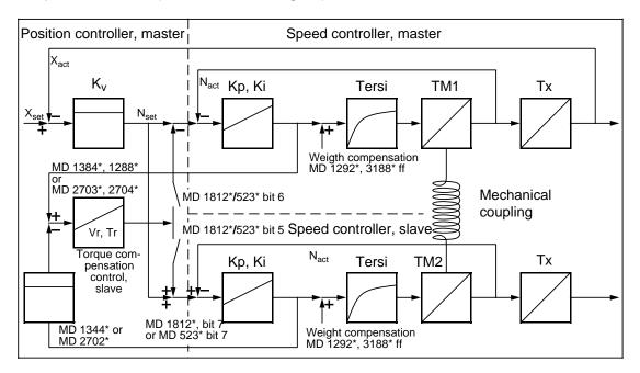
Structure of master/slave with torque compensation control
