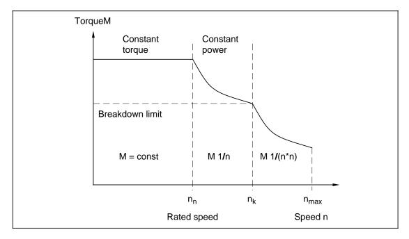
Fig. 1 Torque characteristic of induction motor
