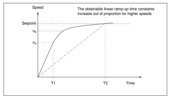
Fig. 2 Speed characteristic during acceleration (thick line)
