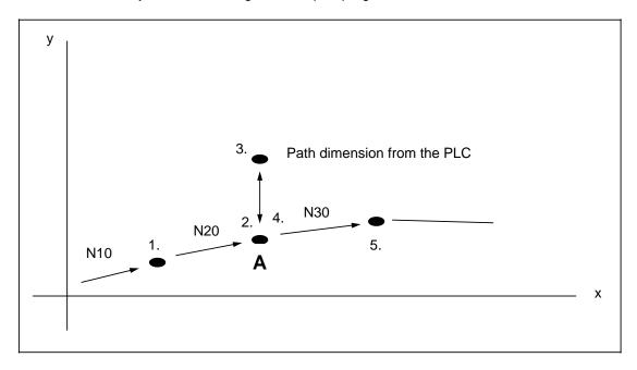
As you can see in the above diagram, the axis positions are corrected to the end point of block N20 (point A) after the path dimension has been traversed and NC start executed. Then block N30 is executed (e.g. with a new tool).
