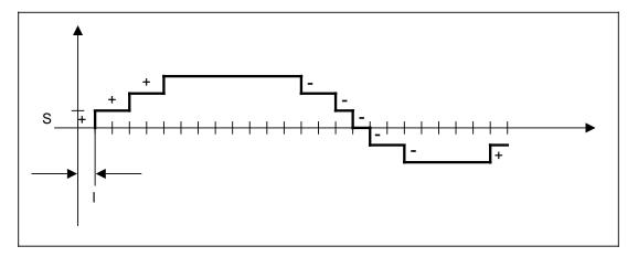
The relevant compensating values for the spacing is based on the permissible tolerance band, and should be selected so that the compensated error curve approximates as closely as possible the ideal condition. The compensating value (0 to 100 units) is transferred to NC MD 328\*.
