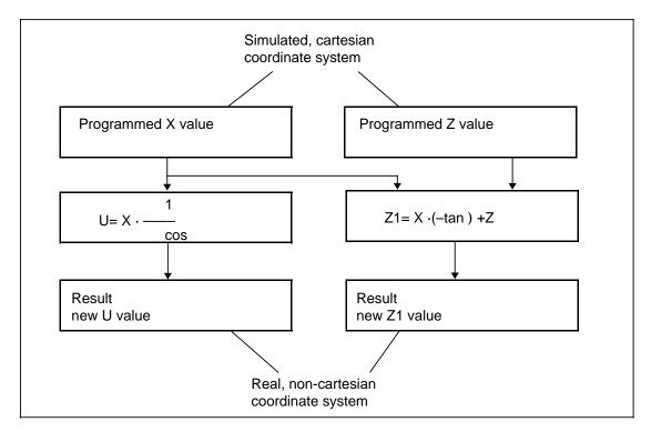
Relationship between the simulated leading axes and the following axes
