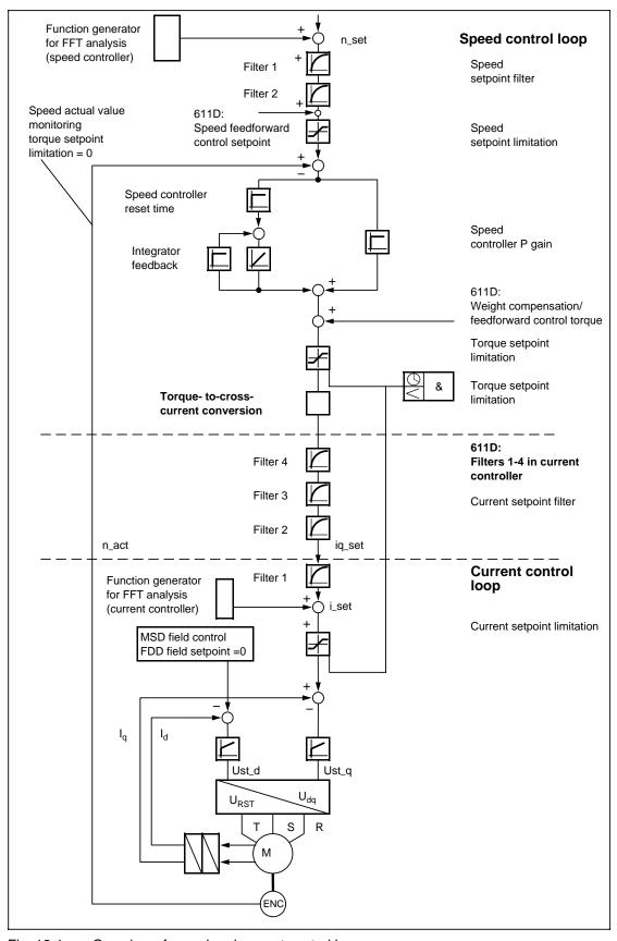
Fig. 12-1 Overview of speed and current control loops
