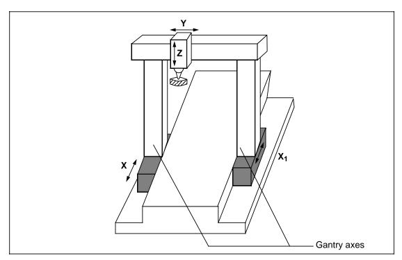
With gantry axes, the two axes should be traversed as one. In addition, only one axis (e.g. X) must be programmed by the user.
