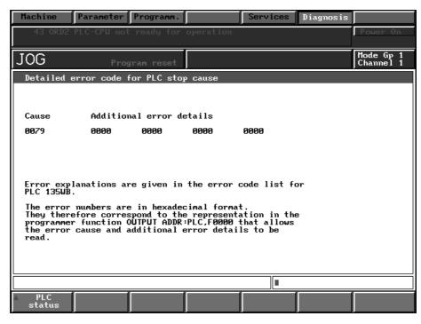
Fig. 3.2 Detailed error code for cause of PLC stop
