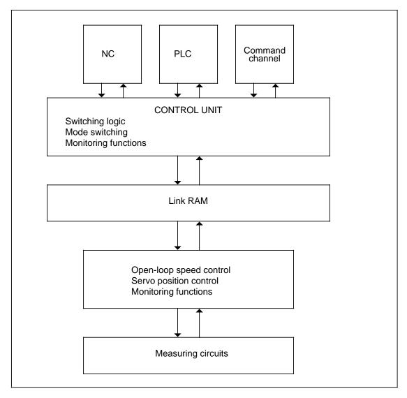
Structure of spindle control
