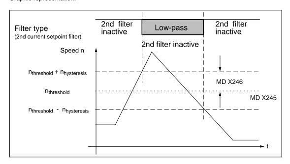
Functionality: The switchover from "Feedthrough" to "Low-pass" takes place when the absolute value of the actual speed exceeds the value  $n_{upper}$  ( $In_{act}I \quad n_{upper}$ ) and vice versa from "Low-pass" to "Feedthrough" when the absolute value of the actual speed drops below the value  $n_{lower}$  ( $In_{act}I < n_{lower}$ ). If the value 0 is entered for the hysteresis, then the two switchover speeds are identical.
