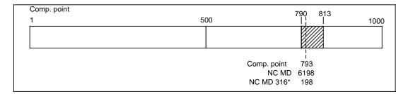
The reference point determines the location of the hatched area of the compensation points used. This area terminates at point 790 or 813 due to the spacing between the leadscrew error compensation points and the maximum traversing range of the axis.
