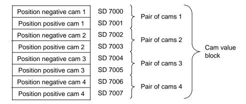
The cam positions must refer to the relevant machine system, in either metric system or inches. They are input into the machine-related actual value system. No check is performed to ensure that the cam positions do not exceed the maximum traversing range.
