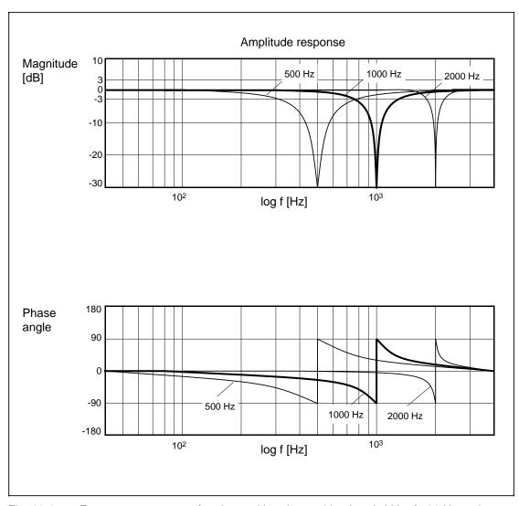
Fig. 12-6 Frequency response of undamped bandstop with a bandwidth of 500 Hz and blocking frequency variations of 500 Hz, 1000 Hz and 2000 Hz.
