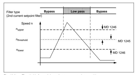
Fig. 12-8 Threshold of speed-dependent torque setpoint smoothing
