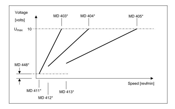
If 3rd gear has been engaged, the new S value must be lower than the contents of MD 413\* in order for the NC to initiate a gear change.
