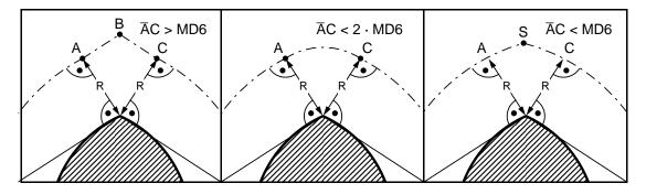
Before switching over, the distance A to C is compared with machine data 6 (MD6). If the distance from A to C is smaller than MD6, the intersection of the two blocks is traversed (applies to all circle transitions with "TRC with transition circle" G450 and "TRC with intersection" G451).
