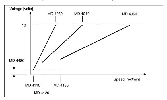
The gear is output on the basis of the lowest switching frequency, i.e. if the speeds of the individual gears overlap, a new gear is output only when the programmed S value is no longer possible for the selected gear.
