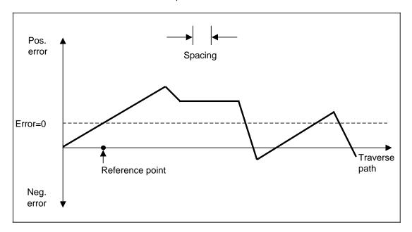
The spacing between 2 leadscrew error compensation points (MD 324\*) is then specified, being based on the permissible tolerance of the final (compensated) leadscrew error curve, the actual leadscrew pitch error and the number of possible compensating values.
