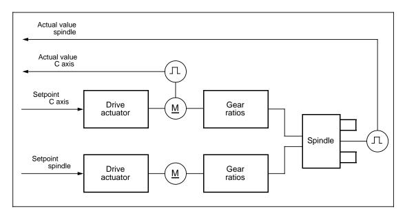
Configuration with two encoders and two drives
