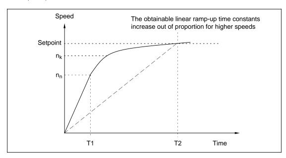
Fig. 2 Speed characteristic during acceleration (thick line)
