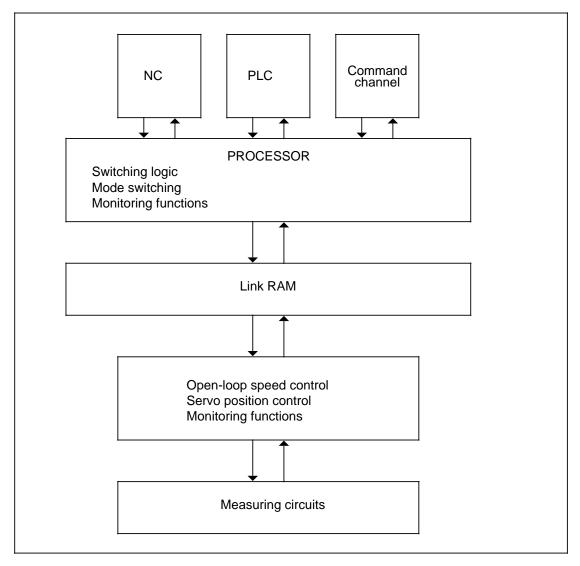
Structure of spindle control
