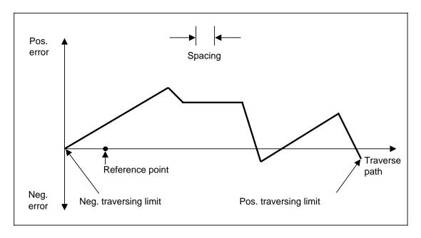
Because compensation is not possible at the reference point, the error curve must be shifted so that the error is zero at the reference point.
