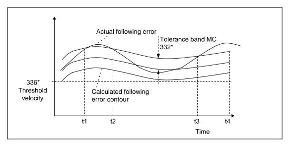
Activating contour monitoring at constant setpoint velocity
