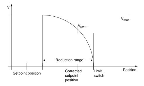
It is possible to define for each individual channel whether or not its path speed must be reduced by means of the PLC signal to channel "Do not reduce channel".
