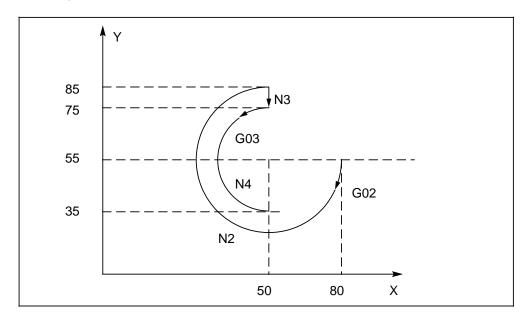
If an interpolation parameter was not programmed because it was "0", the G function, which also precedes the programmed interpolation parameter, also refers to the interpolation parameter that was not programmed.
