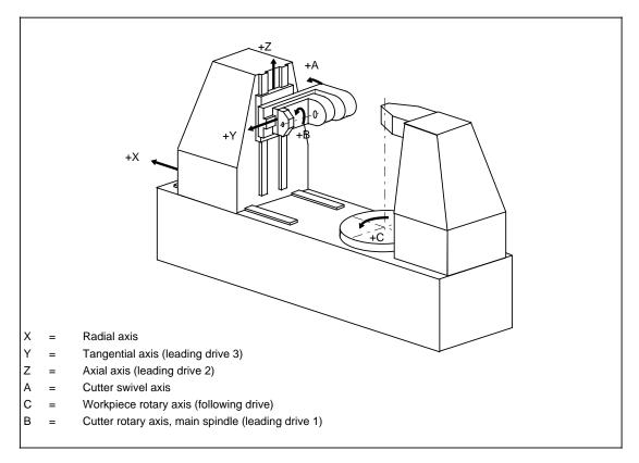
Definition of axes on a hobbing machine (example)
