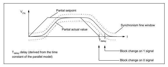
Block change with synchronism fine. Motor operating without disturbance. Behaviour corresponds to parallel model.
