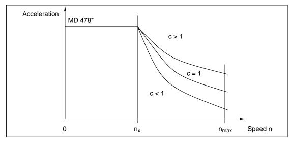
Fig. 3 Possible shapes of acceleration characteristic when adaptation factor is varied. For c = 1 (1 = 100 %), the acceleration above speed limit nx is reduced in inverse proportion to the speed.
