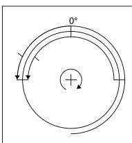
last M19 position: $90^{\circ}$ Actual position: $0^{\circ}$ Specified travel: $-180^{\circ}$
