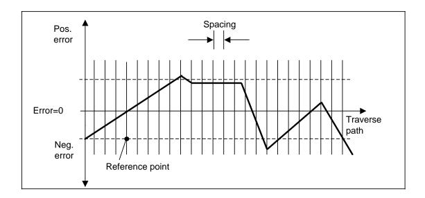
It is then specified how many compensating points must be supplied by means of the entered spacing between 2 leadscrew error compensation points and the end stops at the machine. Since leadscrew error compensation is only active when the axis is synchronized - at the reference point - particular significance is attached to the compensation point coinciding with the reference point. This compensation point is entered in encoded form in MD 316\*. The compensating value at this point must be 0.
