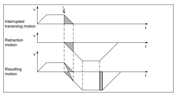
Parameterizable/programmable retraction as open-loop control function
