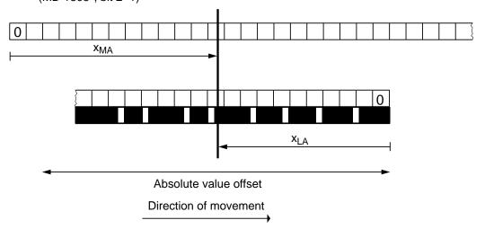
The absolute offset is the offset between machine zero and the 1st reference mark on the linear scale; at any one point (any axis position) the absolute offset corresponds to the difference between the position to be measured in the machine system (e.g. measured with a laser interferometer) and the current position on the linear scale (1st actual value display when MD  $396^* = 0$ ).
