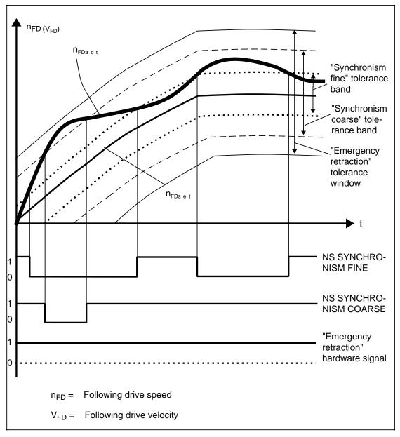
Synchronism monitoring in LINK ON state
