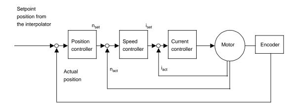
Before the position control system is put into operation, the speed controller and the current controller for the drive must be installed and optimized. When the position control system is installed, the actual position must be checked before the setpoint position is optimized.
