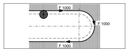
Bit 4 Bit 4=1 The programmed feedrate of the milling tool refers to the tool center path.
