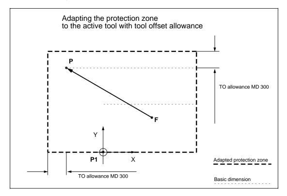
The axes in which the tool offset in the NC channel is calculated and that of the protection zone coordinate that is to be adapted to it are assigned to one another in the axis-specific machine data MD 3938\*.
