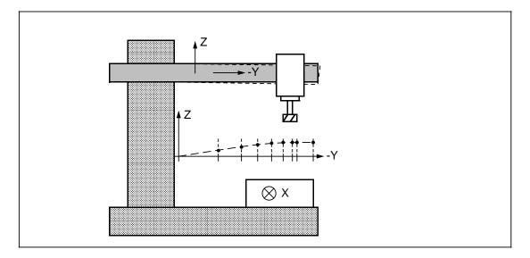
The further the machining head traverses in the negative Y direction, the more the cantilever arm sags in the negative Z direction.
