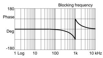
Specified: Blocking frequency 1 kHz with 500 Hz bandwidth 0 Hz bandwidth numerator (damping)
