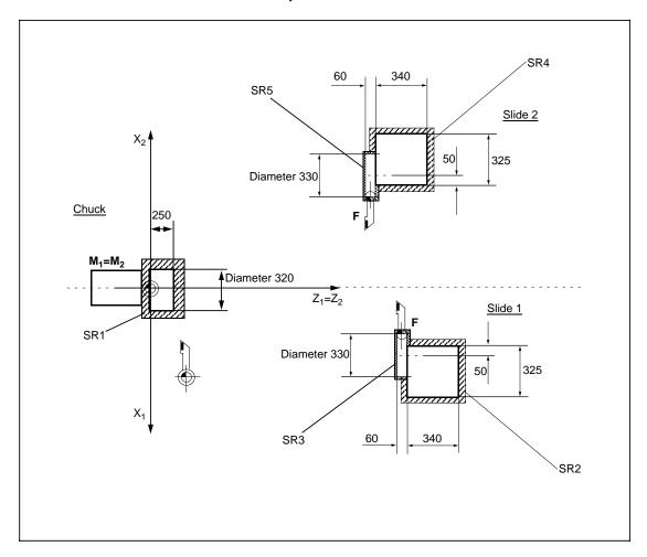
The collision machine data resulting from the dimensions in the example are listed on the following pages.
