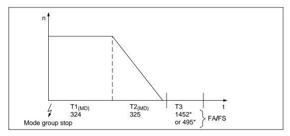
Parameterizable/programmable stop operation as open-loop control function
