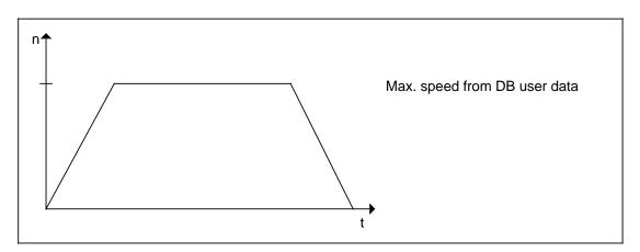
Speed characteristic for incremental positioning
