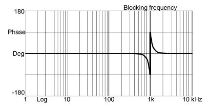
Specified: Blocking frequency 1 kHz, 500 Hz bandwidth and 250 Hz bandwidth numerator (damping)
