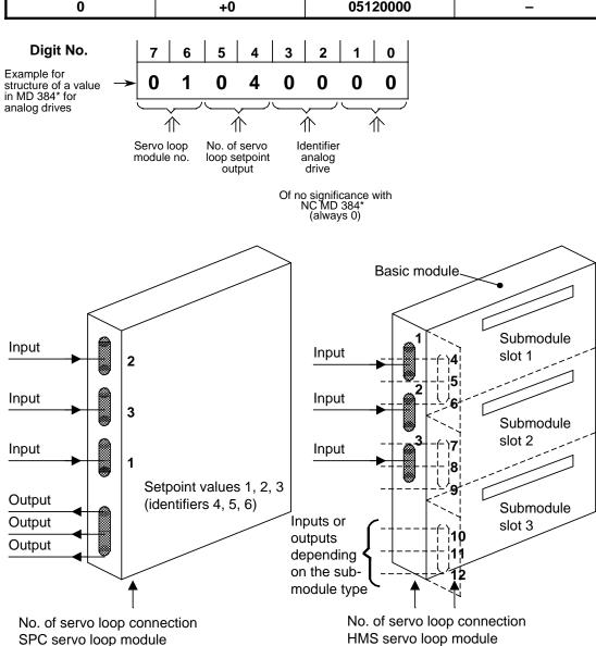
MD 384\* determines at which servo loop module or which output the axis setpoint values are output (see also NC MD 200\*).
