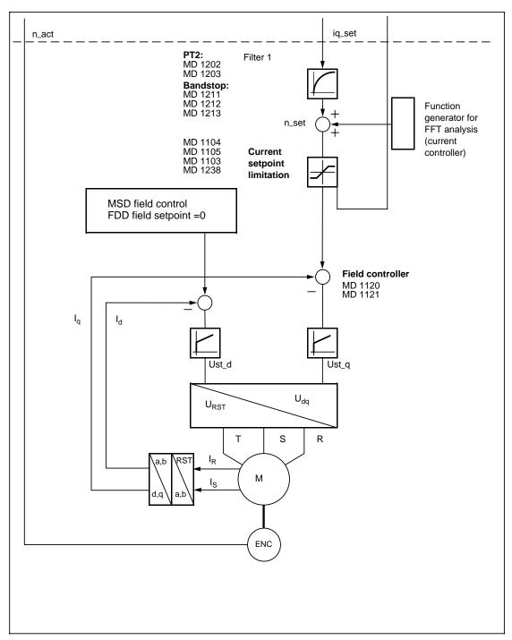
Fig. 12-3 Overview of current control loop
