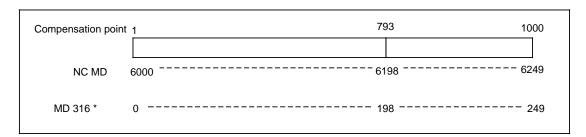
In view of the fact that the SINUMERIK 840C has a total of 1000 compensation points for all axes, the control must be informed via MD 316\* as to which of these 1000 points corresponds to the axis reference point. The compensation point is not entered directly in MD 316\*, the MD offset (MD 6125 = MD offset = 125) being entered instead, so the reference point can only be located on compensation points 1, 5, 9, 13, 17, ... .
