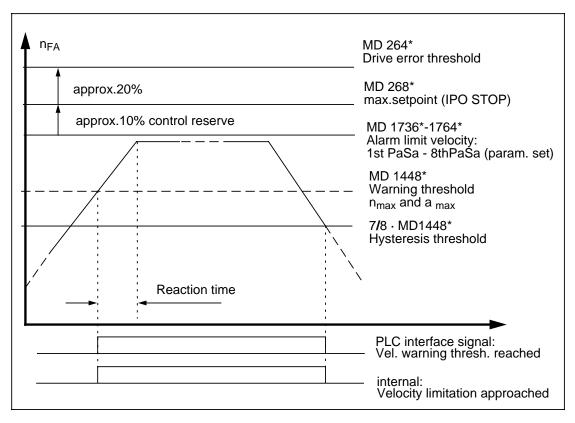
Characteristic of the velocity setpoint with the characteristic rising above and falling below the warning threshold
