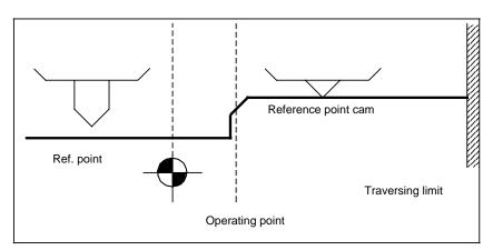
Bit 6 = 0If the axis is between the reference point cam and EMERGENCY STOP when the control is powered up, the axis moves to EMERGENCY STOP during reference point approach, as the control cannot detect from the "Deceleration" interface signal whether the axis is ahead of or behind the reference point cam (also see Section Axis (Analog) and Spindle Installation).
