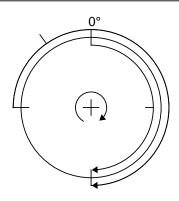
Last M19 position:  $0^{\circ}$  Actual position:  $270^{\circ}$  Specified travel:  $+180^{\circ}$
