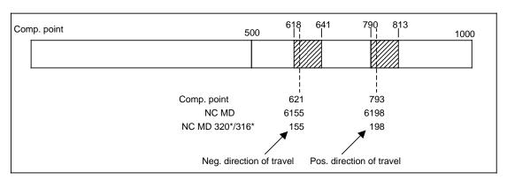
Both direction-dependent and direction-independent leadscrew error compensation are options, and must therefore be ordered. MD modifications do not go into force until after POWER ON and reference point approach. Because the compensating value at the compensation point must be processed as quickly as possible, the specified acceleration value (NC MD 276\*) is not applicable in this case.
