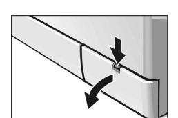
This is necessary if the washing solution cannot be completely drained. The pump is blocked by either loose debris or fluff which accumulates if fluff-giving fabrics are washed at high temperatures.
