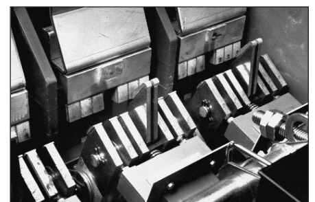
Main and Arcing Contacts — Similar Design for all Ratings
