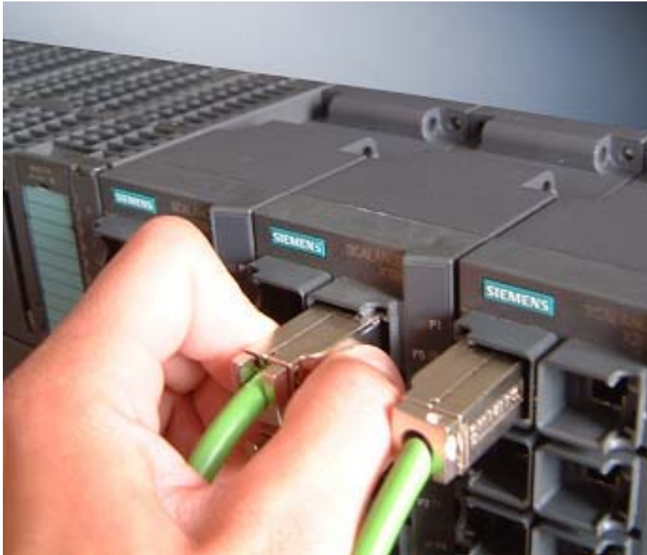
Figure 5-6 Unlatching the RJ-45 plug
