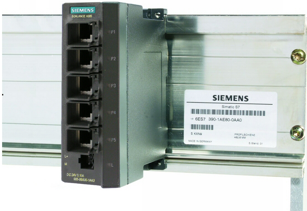
Figure 5-3 SCALANCE X005 installation on a SIMATIC S7-300 standard rail
