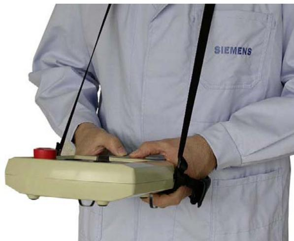
The hand holding the HMI device can also be used to activate the enabling button. The enabling button is optimally accessible. In a dangerous situation, a safety shutdown is triggered in a panic reaction by releasing or fully pressing the enabling button.
