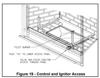
burner and pilot burner area for dust or carbon build-up. This may be removed from the burner or logs with a soft bristle brush. A visual inspection of the pilot burner and main burner flame should be performed to verify proper operation, refer to operating instructions for proper adjustment. Care should be taken when cleaning and handling logs since they become brittle with use. Small heat cracks in the logs do not affect the operation of the log set.
