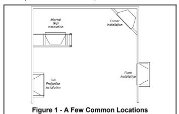
A <u>flush installation</u> is recommended where space is limited or at a premium. Check local codes for any restrictions.
