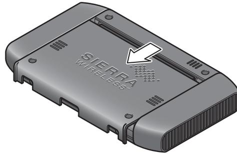
2. Slide the SIM card holder to the **Open** position.
