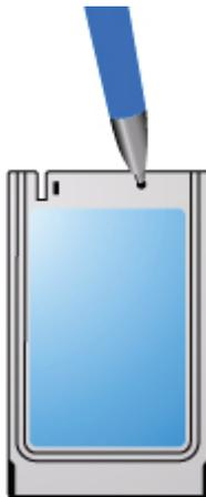
Figure 2-3: Ejecting the SIM card
