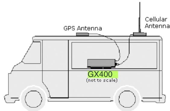
Figure 3-3: GPS Antenna Placement for a Vehicle
