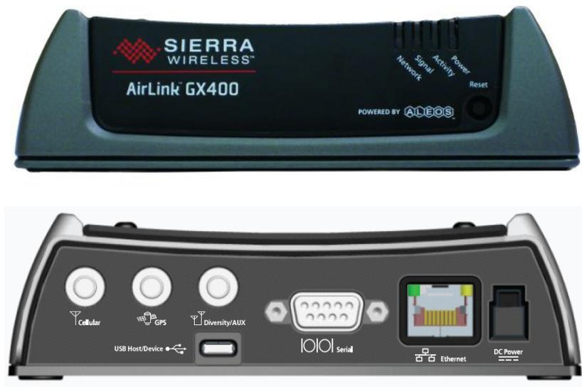
Figure 3-1: AirLink GX400 front and back plates
