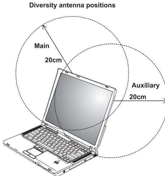
**Note:** The transmission diversity function is implemented for the models: WM3B2200BG, WM3B2915ABG, and AR5BMB-44. The function does not emit radio frequencies simultaneously from both antennas. One of the antennas is selected automatically or manually (by users) to have good quality of radiocommunication.
