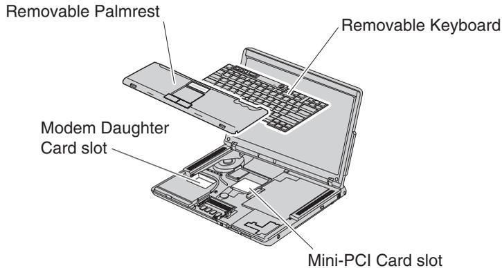
**Attention:** The ThinkPad Z60m Series computer contains an authentication mechanism. If you install an unauthorized wireless LAN Mini-PCI Card that is not approved for use in the ThinkPad Z60m Series computer, the computer will not start, but only displays an error message and emits beeps.
