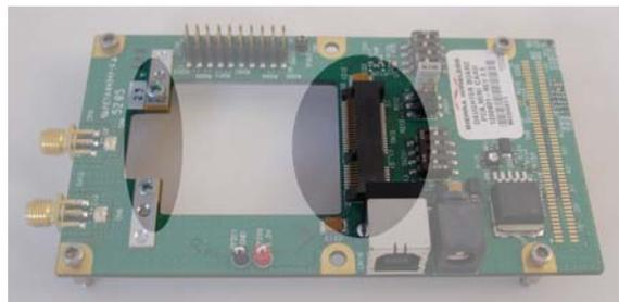
2. Remove the two screws that are located on the metal strips near the antenna end of the board.
