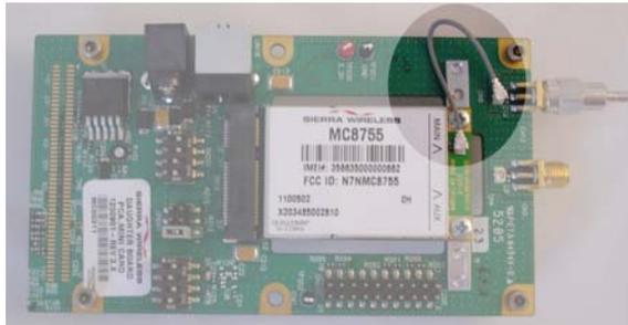
4. Connect the antenna to the adapter. (The first few times you attach the antenna, it may be quite snug.)
