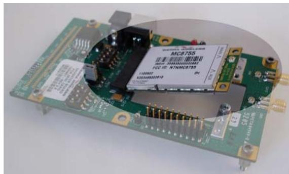
4. Push and hold the module down when it is firmly seated in the slot and then fasten it using the screws removed in Step 2.
