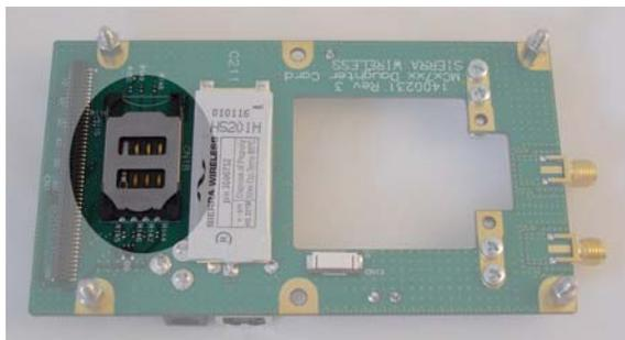
2. Open the USIM casing – the casing latches in place, so you may have to push the tab marked “LIFT” slightly to the side before lifting it.
