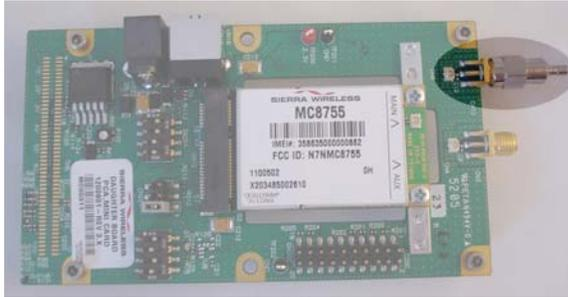
3. Connect the Mini Card's main antenna to the daughterboard's main antenna connector using the gray wire provided – press down lightly on the connector ends (the first few times you use these connectors, they may be quite snug – press straight down on the end to get a secure connection).
