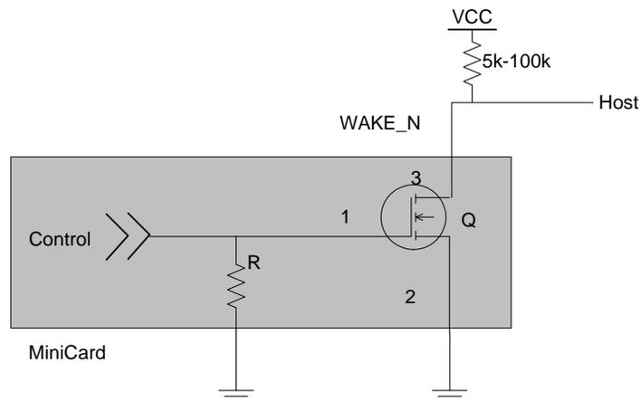
Figure 3-4: Recommended WAKE\_N Connection
