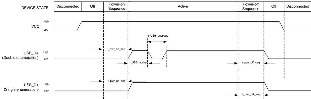
Figure 5-1: Signal Timing (USB Enumeration)
